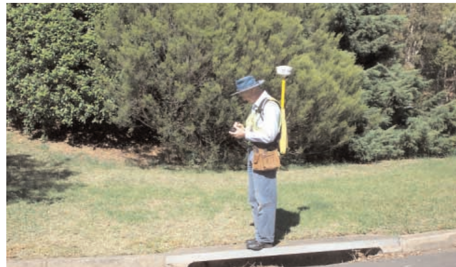
Garth Graham is a surveyor employed by Baulkham Hills Shire Council to collect GPS data on their drainage system for the flood studies
